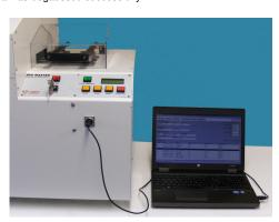
If this data is highlighted and the print button pressed all the details on the screen along with all the data entered will be printed as a report. As new media is erased the details will be added to the Media Processed Log in the lower half of the screen. By highlighting erase records, the logs of one or more can be printed as required,
